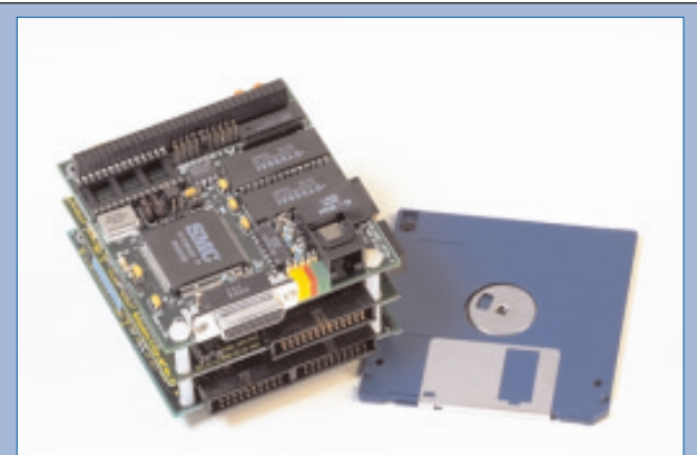
A PC/104 system component is about the same size as a 3.5-inch diskette.
